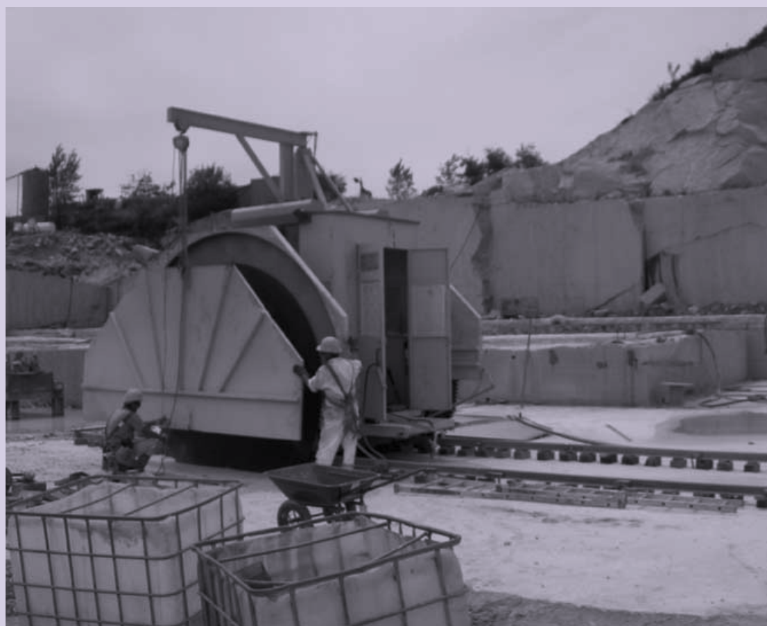
EXTRACTING STONE FROM THE TARN QUARRY (FRANCE) 'CUT TO ORDER' RATHER THAN CRUDELY BLASTED FROM THE ROCK FACE. THE PARAMETRIC MODEL OF THE NARTHEX COLONNADE GENERATES 3D MODELS FOR THE GRANITE BLOCKS IN ORDER TO MINIMIZE WASTE.
